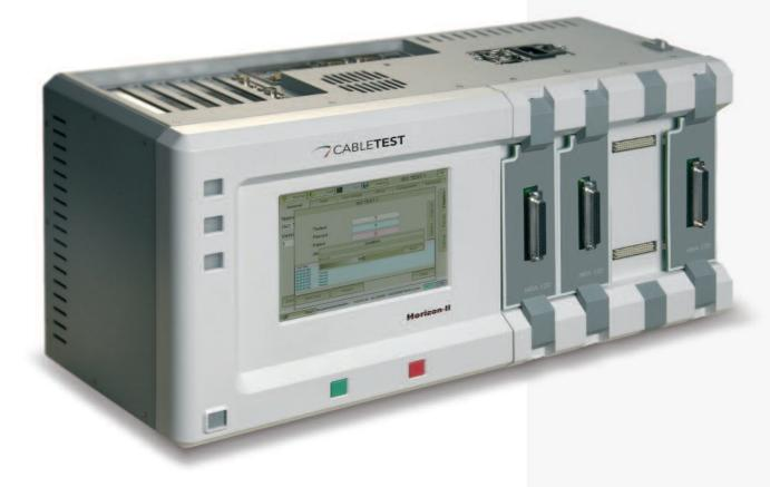
The Horizon II bench top wiring analyser enables 128-point cable testing with modular expansion capability up to 1024 points capable of performing continuity and dielectric strength testing up to 1500V DC and/or 1067V AC. The Horizon II has a vast range of optional connection plates available for the most common types of cable interfaces.
