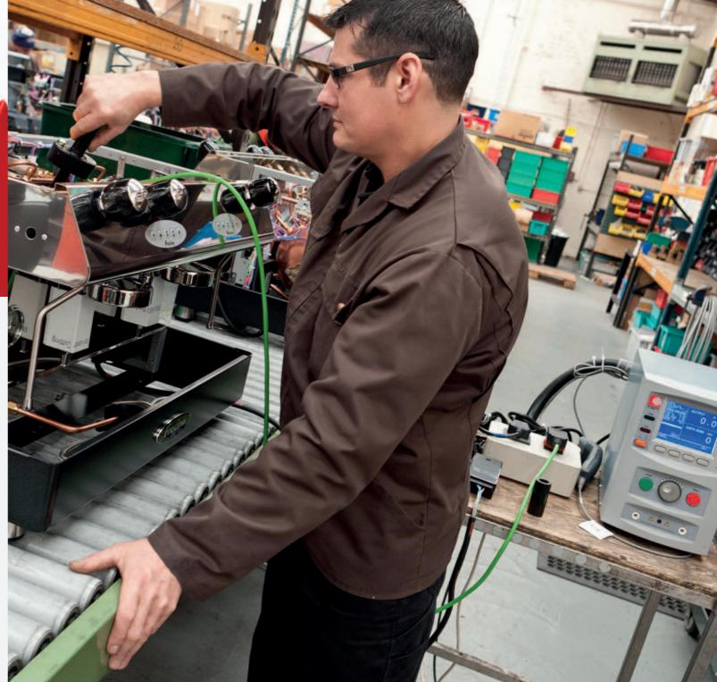
Fracino use the advanced, multi-function HAL 104 to test product reliability, to ensure they operate correctly and to the highest standard in performance and safety. It's a fast and efficient automatic manufacturing solution.
